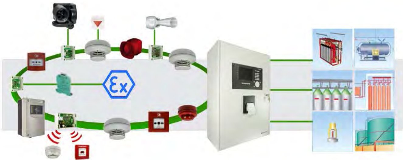
Fig. 24 Topology of a SecuriFire ECP / FEP 3000
