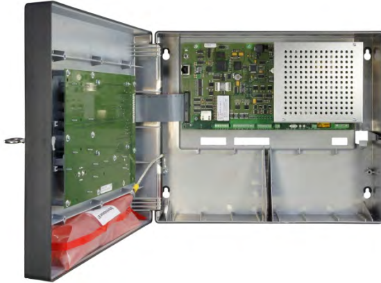
Fig. 60 Basic circuit board with PSU and integrated MIC
