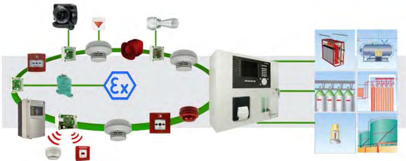
Fig. 25 Topology of a SecuriFire ECP / FEP 2000 control panel
