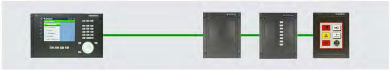
Fig. 27 Schematic of an EPI-BUS
