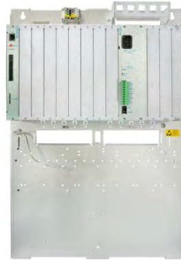
Fig. 54 Main control unit fitted with boards
