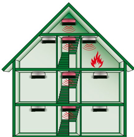
Fig. 7 Collective alarm line (example: fire in an apartment building)
